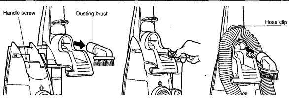
1) Remove the dusting brush from the handle and align it with the body of the cleaner in the proper position as shown in the illustration.
